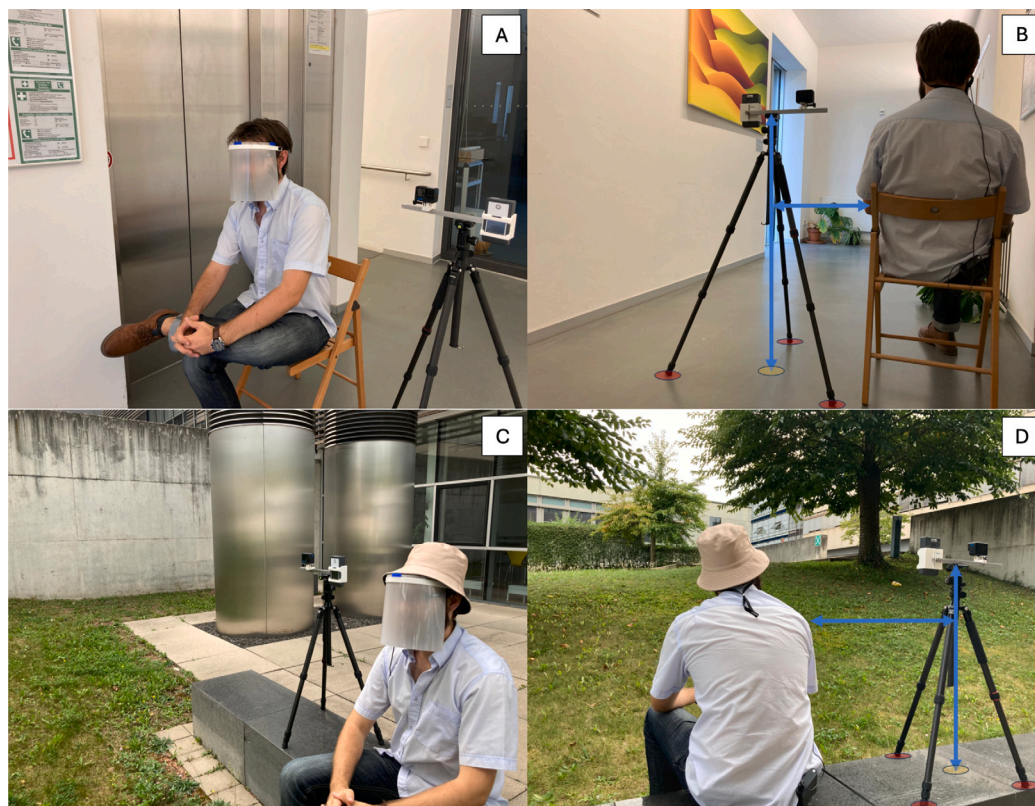
Fig. 3. Example of the setup and a participant in IME 2 (A & B) and OME 1 (C & D). Panels A and C show the participant during the light-adaptation phase, during which the face shield preserved retinal adaptation while diffusing scene details. Panels B and D show the measurement itself. In outdoor measurement environments, participants wore a hat to shield themselves and the eye tracker from direct sunlight. The blue arrows and red circles on the ground indicate standardized distances and positions.
