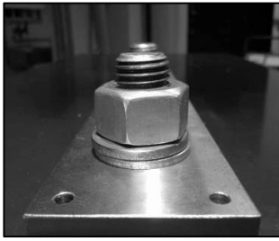
Fig. 12. Two washers error scenario. The second washer will cause an error detection within Stage 3 or 4, since the desired angular position of the nut will not be reached.
