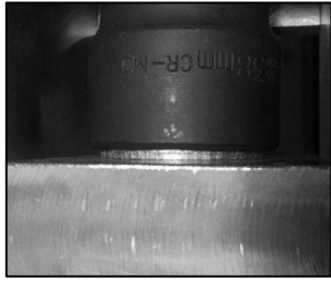
Fig. 13. Missing nut scenario: the tool is touching the washer as soon as it is placed on the nut, because of the missing nut.
