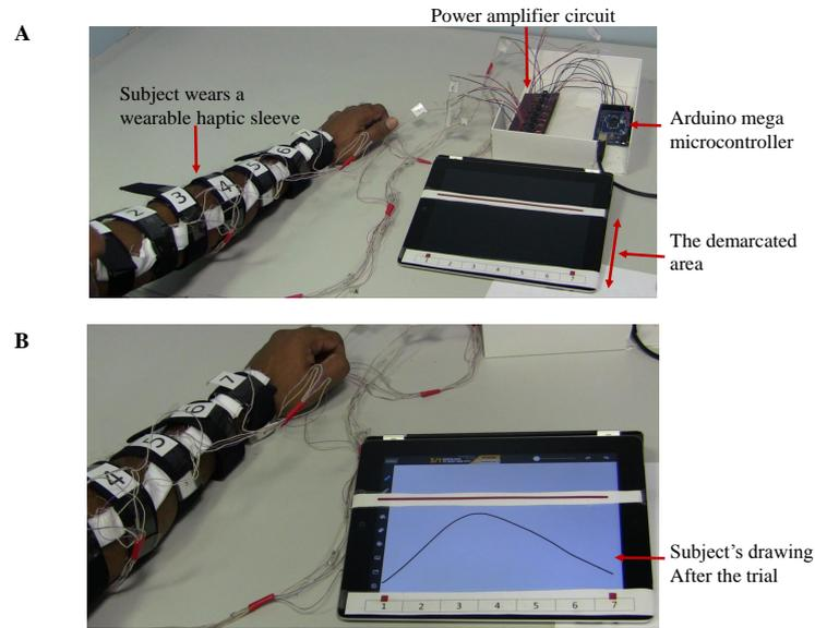
**Fig. 2.** An experimental trial: A) The subjects wear a wearable haptic sleeve with 7 Pico Vibe 10 mm vibration motor. The drawing area is demarcated and used hardware is shown, and B) The subject drew the intensity felt from the vibro-tactile actuator arrays was during the trial on iPad demarcated area. Draw free app (Apple Inc) software is used as a drawing tool.
