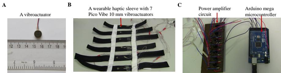
**Fig. 1.** Hardware design for wearable haptic sleeve: A) Pico Vibe 10 mm vibro-actuator, B) A wearable vibro-tactile actuator arrays with 7 Pico Vibe 10 mm vibro-actuator motors, and C) Arduino Mega motherboard and power amplifier circuit to generate different intensity patterns.
